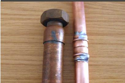
22mm pipe with lead solder and 15mm pipe with lead free solder
