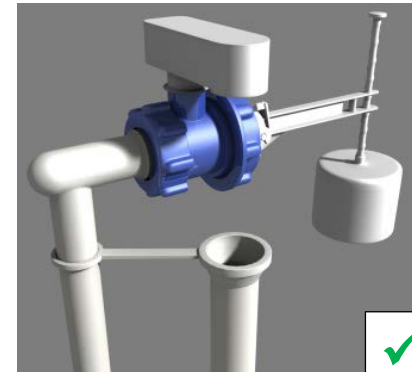
Fig 6: Example of a silencer tube which does not compromise the air gap
