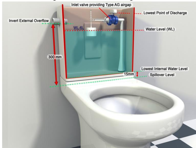
Fig 2: internal overflow arrangement
