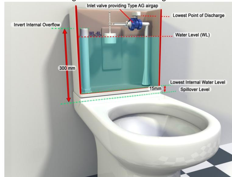
3. Is the measurement between the spillover level of the WC (receiving vessel) and the invert<sup>3</sup> of the warning pipe at least 300mm?
